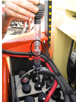
Figure 6-8. Measuring Electrolyte Specific Gravity
